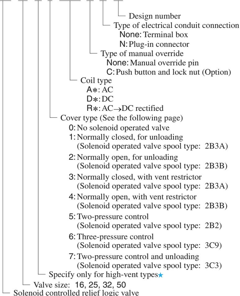
★ Use high-vent pressure types if the shifting time from unloading to on-loading is reduced.
