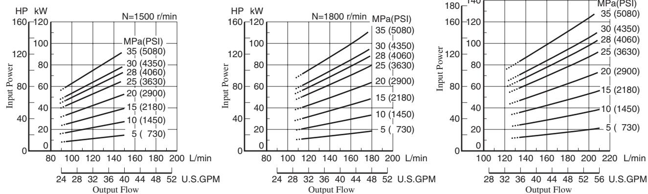
Note) The dotted line in the graph indicates less than minimum adjustable flow.
