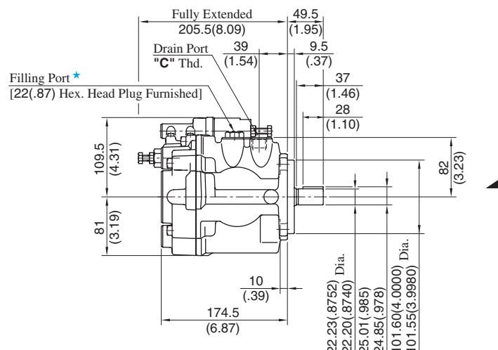
★ Install the pump so that the "Filling port" is at the top.
