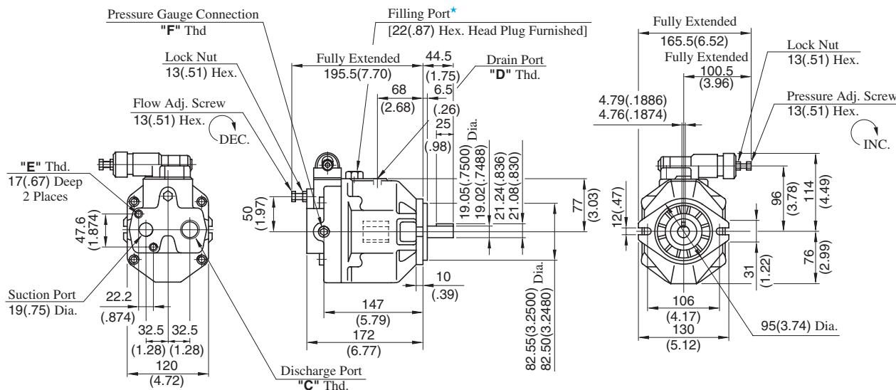
\* Install the pump so that the "Filling port" is at the top.
