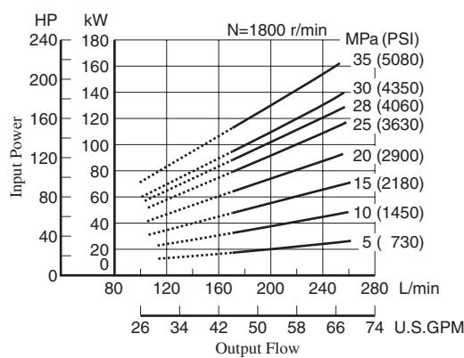
Note) The dotted line in the graph indicates less than minimum adjustable flow.
