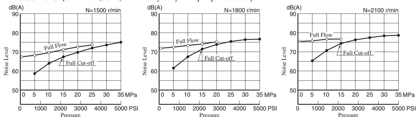
Typical Performance Characteristics of Type "A3H145" at Viscosity 32 mm<sup>2</sup>/s (150 SSU) [ISO VG32 oils, 40°C (104°F)]
