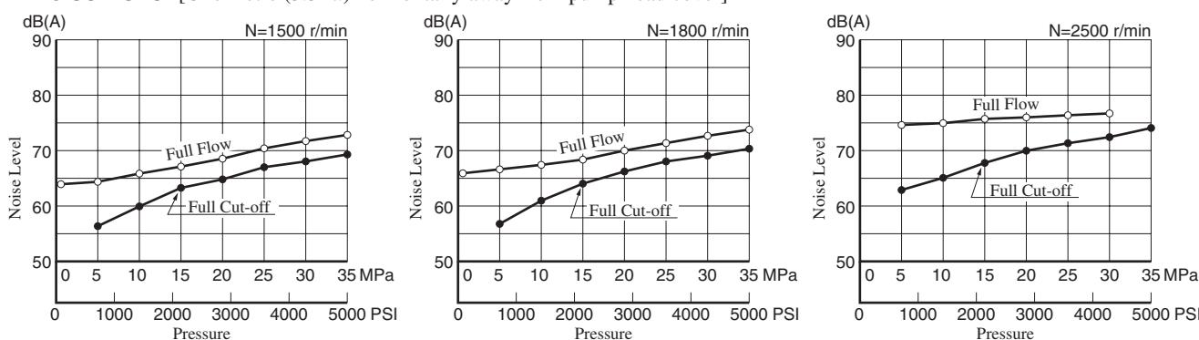
Typical Performance Characteristics of Type "A3H71" at Viscosity 32 mm<sup>2</sup>/s (150 SSU) [ISO VG32 oils, 40°C (104°F)]
