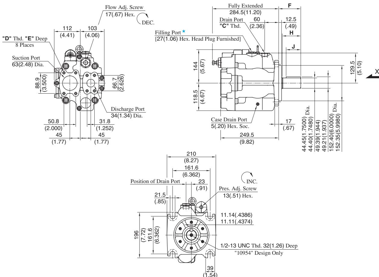
★ Install the pump so that the "Filling port" is at the top.
