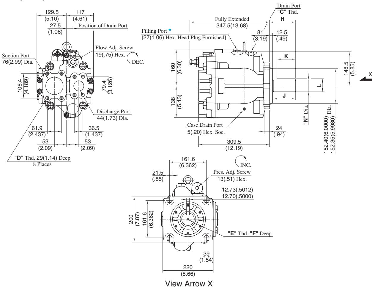
★ Install the pump so that the "Filling port" is at the top.
