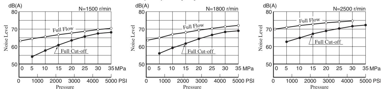
Typical Performance Characteristics of Type "A3H56" at Viscosity 32 mm<sup>2</sup>/s (150 SSU) [ISO VG32 oils, 40°C (104°F)]
