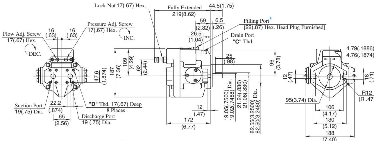
\* Install the pump so that the "Filling Port" is at the top.
