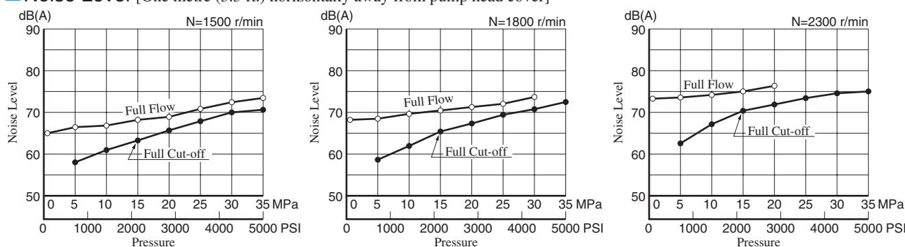
Typical Performance Characteristics of Type "A3H100" at Viscosity 32 mm<sup>2</sup>/s (150 SSU) [ISO VG32 oils, 40°C (104°F)]
