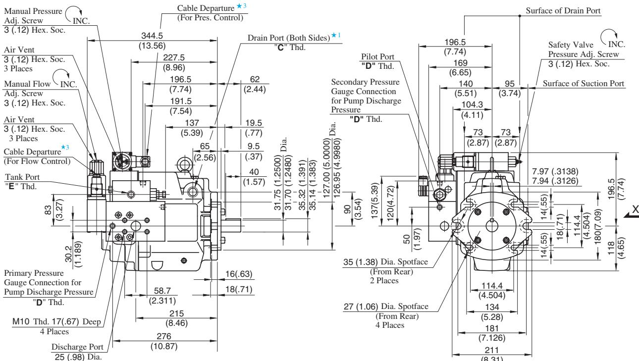
★ 1. Use either port or two drain ports at your option. Keep the remaining port plugged.
